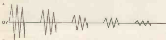
Fig. 1 (above). A combination of the signal's natural decay characteristic and the "chopping" effect of the unit gives an "echo" effect output signal.
