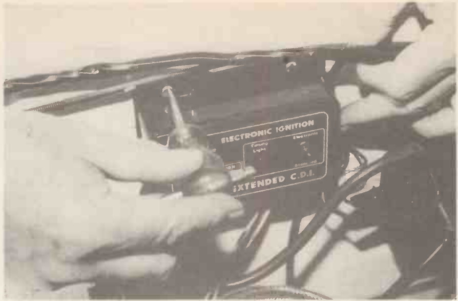
With the kit assembled, fitting is very straightforward, using the three self-tapping screws supplied. The unit is easily wired into the ignition circuit.
