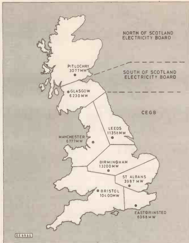
Fig. 10. Grid control centres.
