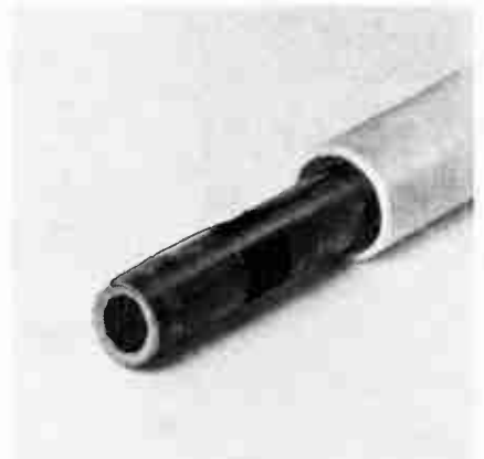
The search coil constructed from 250 turns of 30 s.w.g. with the ferrite rod positioned in cardboard former.
