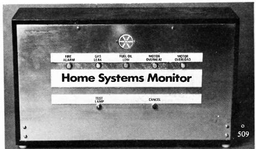
The Home Systems Monitor unit (below) with front panel labelled to show the monitored functions.
