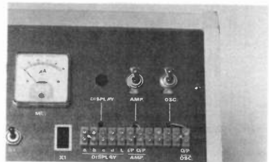
Minilab from panel showing the amplifier section.
