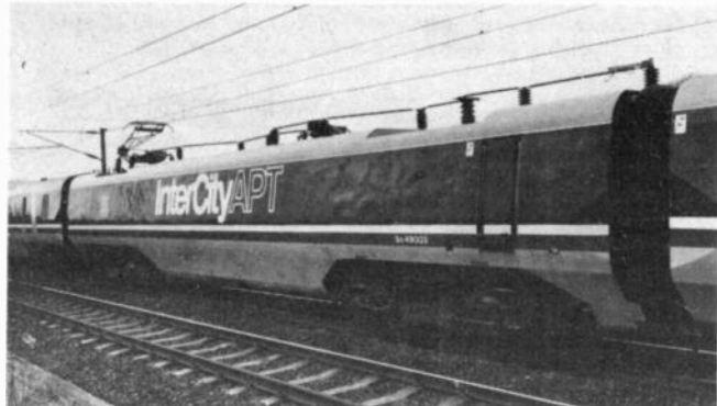
The prototype 4000hp Power Car contains most of the monitoring equipment, power equipment and braking and tilt sensing equipment. It is hoped to fit this into a driving power car including the driving cab.
