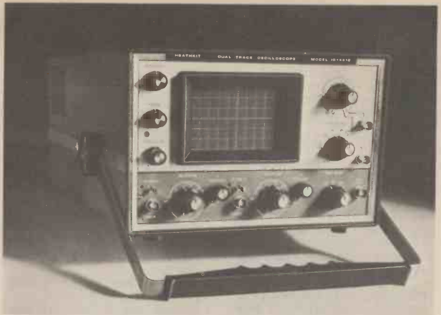
Typical of many oscilloscopes, is the facility to provide two traces. The IO-4510 from Heathkit is a good example.
