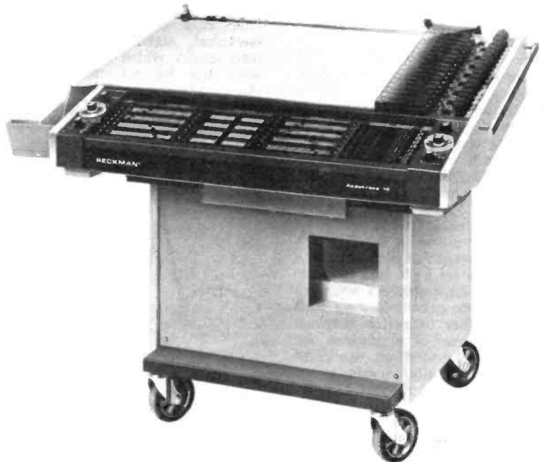
The Beckmann Accutrace—a modern electroencephalograph.
