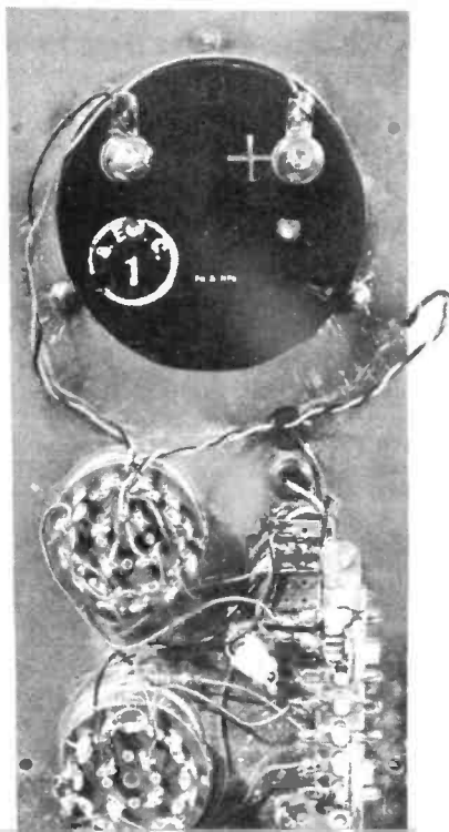
Fig. 2. Layout and wiring of the Transistor Checker. Fig.3 (Right). Test arrangement.
