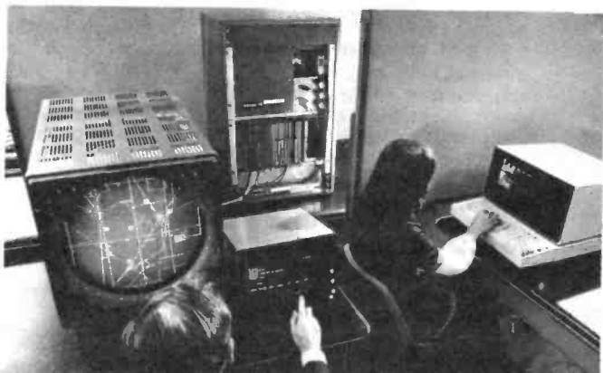
Latest air traffic control radar display by Marconi Radar. The control computer for distributing the radar data is centre background.
