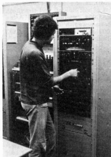
A student from the Cayman Islands, operating a submarine cable test set at Porthcurno.
