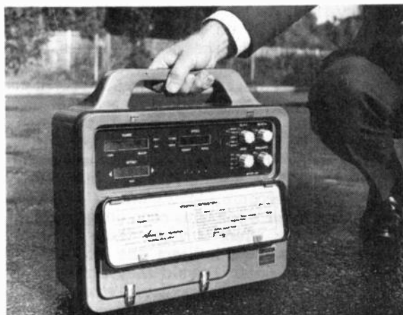
The Decca Channel Approach Aid. Weighing 22lbs, and transported in a waterproof covering this is taken aboard with the pilot. At Milford Haven it functions in co-operation with one of three shore beacons, as selected, to provide speed, distance to any pre-determined point and distance offset either side of the leadline. The Aid is entirely independent of any other system and incorporates its own batteries.
