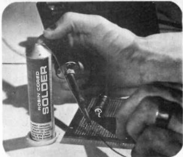
Soldering a transistor to Veropins using pliers as a heat shunt.
