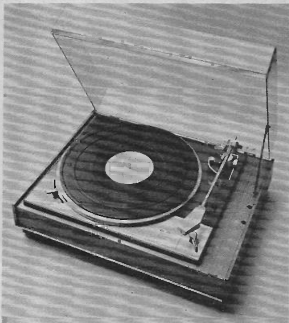
Photograph of a Goldring-Lenco turntable, type GL75 with variable speed control.
