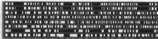
Figure 11: an illustration of the "human bar code" or IrisCode generated for digital storage and later comparison
