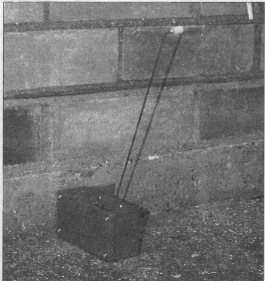
Photo 4: the sensor box showing the angle of lean, right-angled upper end (make sure it is pointing the right way when the sensor is threaded into its pot), and plastic buffer on the wire tip
