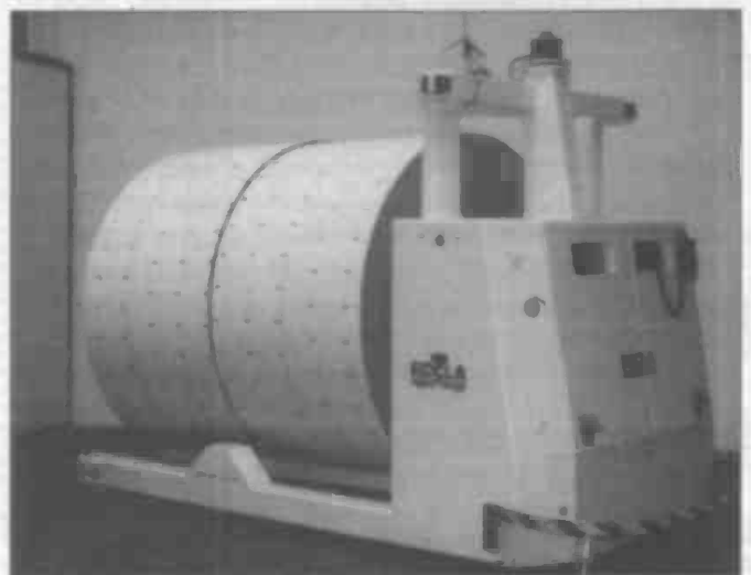
An AGV (Automatically Guided Vehicle) transporting paper rolls automatically in a factory environment. Note the hand-held pendant on the right, used for controlling the AGV manually. (Picture courtesy of Rocla (Finland)/Mentor (USA).)
