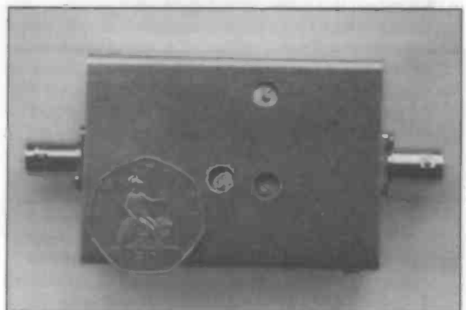
The filter boxed, showing the three trimmers and an old-style 50pF coin for comparison!
