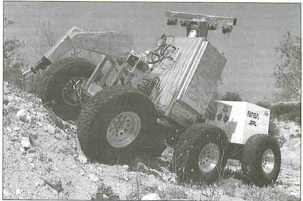
Figure 15 View of prototype rover 'Robbie' - a considerably more massive vehicle weighing 2 tonnes (Courtesy NASA)
