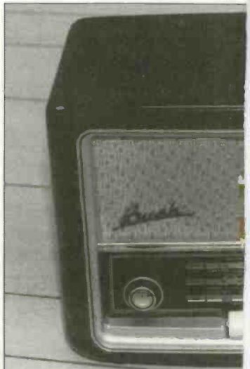
The Bush DAC10. This set covers MW preset tuning. It was released in 1950
