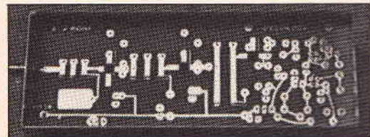
2.0-2.6GHz Signal source using microstrip PCB circuit board
