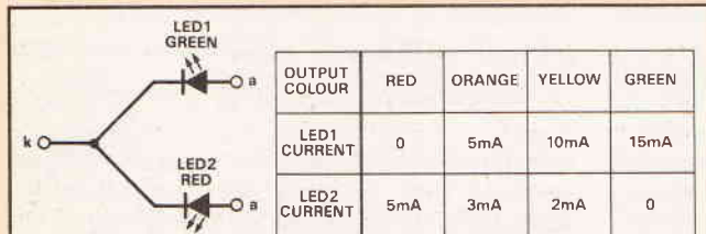
Fig. 10 'Multicolour' LED, giving four colours from two junctions
