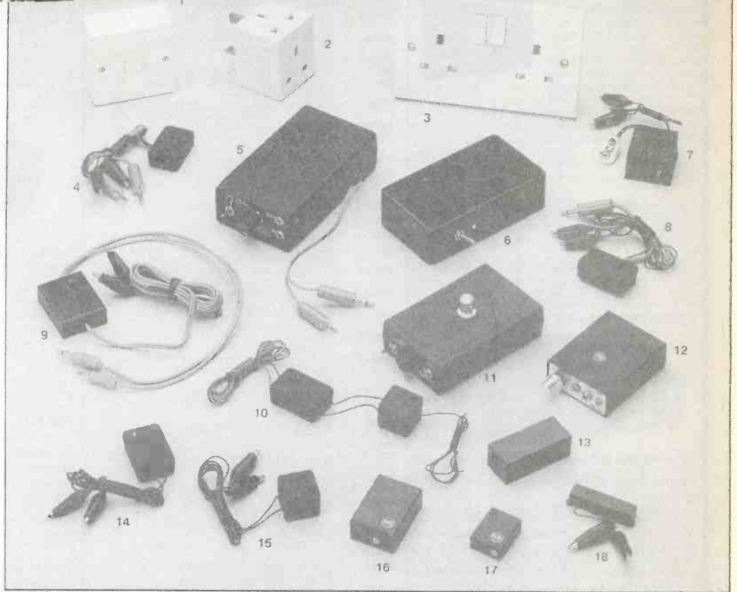
A selection of off-the-shelf surveillance equipment available from Lorraine Electronics Surveillance. 1-3 discreet transmitter housings; 4,8,9,13-15,18 telephone surveillance devices; 5,12 amplifiers; 6,7,10,11,16,17 transmitters.
