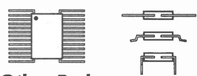
Fig. 3 Size comparison of DIL and various surface mounting devices.
