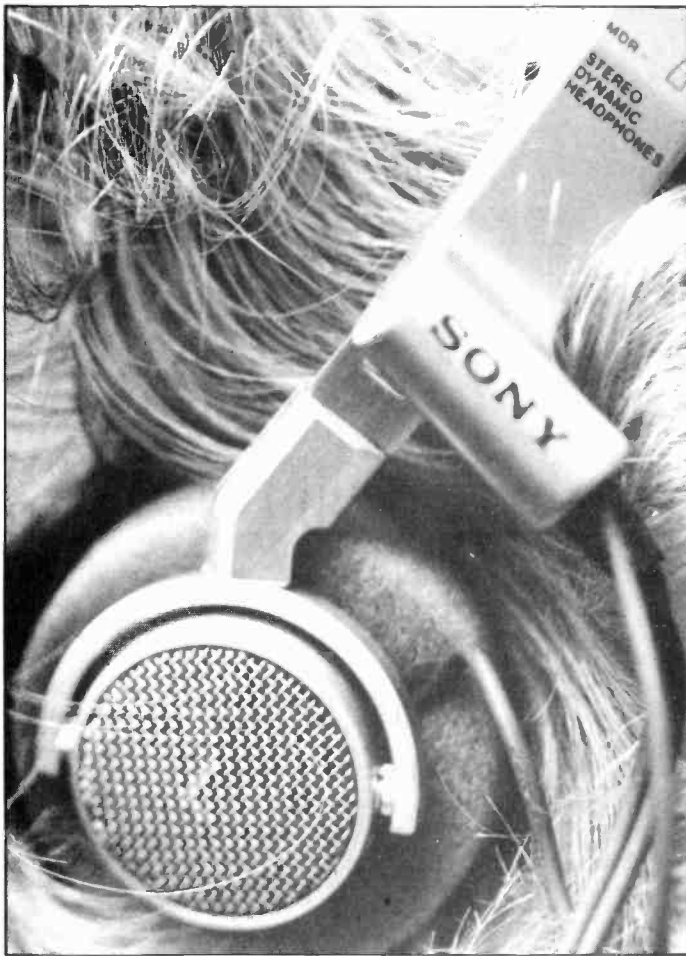
Above: The MDR-7 in use. Only one earpiece is adjustable, the other being fixed to a swivel joint to better align with the user's head. Cable entry is side-on and much more convenient than on the MDR-3 where it hangs awkwardly, stethoscope-like, behind the ear pieces.
