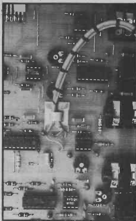
Close-up showing the wiring to Molex connector 'A' (on the input board).
