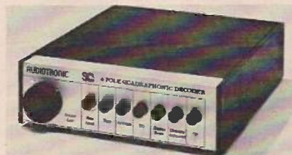
Audiotronic 6-pole remote control SQ decoder for 4 channel discs and tapes.
