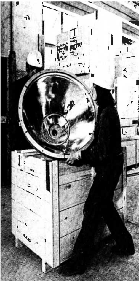
Seen here is one of the 550 metal halide vapor lamps used in the main stadium. Each lamp draws 28 kW.
