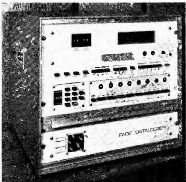
PACE Data logger from EAI scans to 100 channels/sec. and is accurate to \pm 0.05\% .
