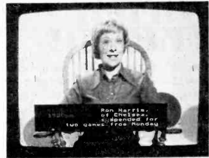
A major attraction of Teletext is likely to be the Newsflash. Receivers will probably be designed to enable the viewer to choose for Newsflashes to be superimposed on a regular programme either in a box as shown or in white.
