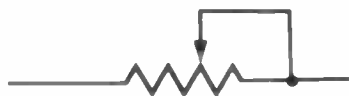
Fig. 6. Pots in some applications require only a variation in resistance. Which terminals are connected together depends on the circuit effect.
