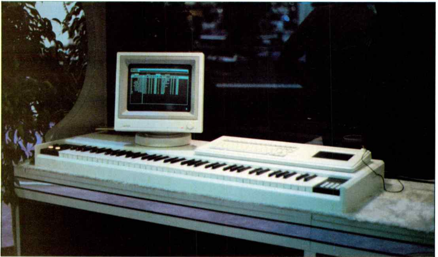
Fairlight Series III has 16-bit polyphonic sampling now, completely updated software and data
