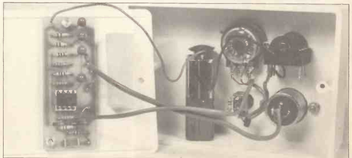
Internal view of the D.I. box.
