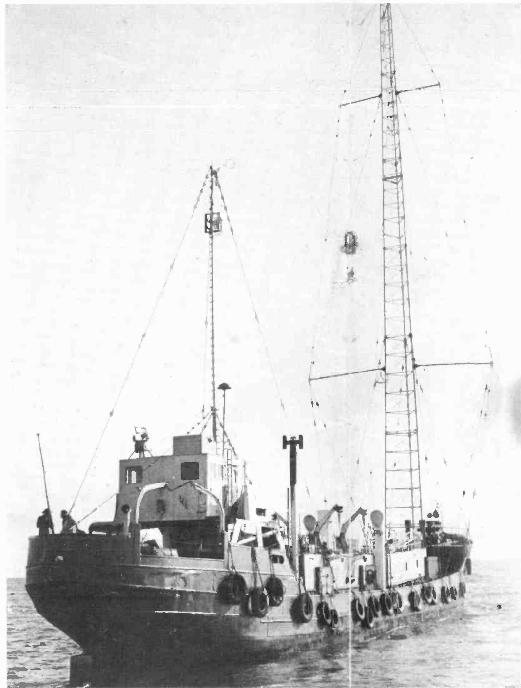
Mi Amigo - June 1973, clearly showing the new vertical aerial mast and the horizontal aerial. (courtesy FRC Holland)
