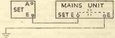
FIG. 12.—Essential safety condenser for the earth connection of a D.C. mains unit.
