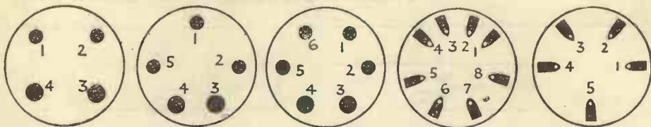
These bases are (left to right) four, five and six pin Continental types, and the "P" and "V" type Mullard universal side-contact bases, respectively.
