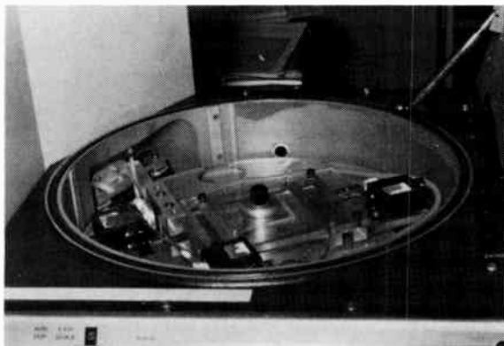
Fig. 4. A device for remote sample positioning in the x-ray fluorescence spectrometer
