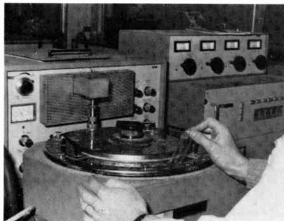
Fig. 1. Automated gas chromatography equipment for alcohol analysis.
