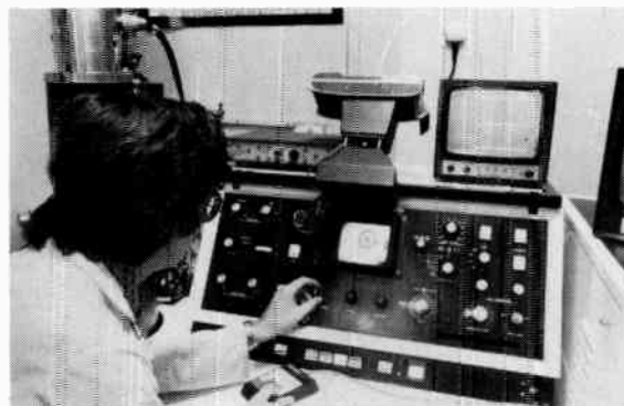
Fig. 5. Scanning electron microscope equipped with microprobe analyser
