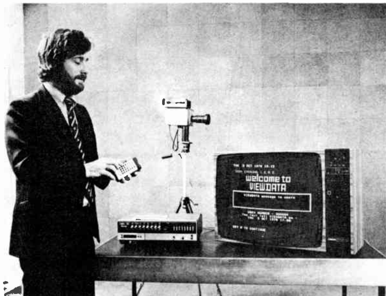
Fig. 1. Modern 26-inch colour television receiver incorporating Teletext and Viewdata with video cassette recorder and home colour camera, as demonstrated.
