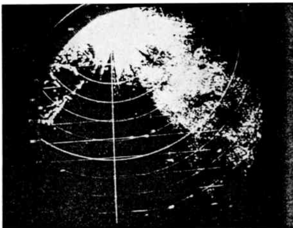
Fig. 12. Rain and sea clutter at a coastal radar site. Notes: (i) No anti-clutter measures employed. (ii) 0.5 n.m. range rings. (iii) Three buoys shown SSE at 3 n.m. (iv) At around 1 mile rain and sea clutter merge. 19th April 1970.
