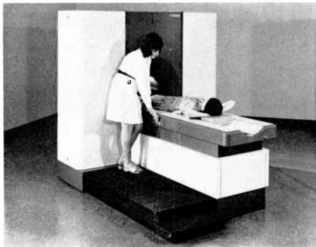
Fig. 2. The EMI Body Scanner.
