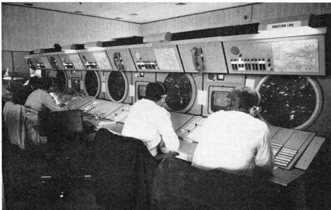
Part of the air-traffic control room at Eurocontrol, Maastricht. Primary and secondary radar information employing an extensive computer complex is used to maintain direct radio contact with aircraft over Northern Europe. Eurocontrol controls civil aviation air traffic only above the 6000 m (20 000 ft) limit in the air space over Belgium and Luxembourg. In the near future, this Maastricht control centre will also be in charge of air traffic over Northern Germany, Holland and part of the North Sea. Decca, Plessey and other British firms have supplied equipment for various parts of the Eurocontrol organization; air conditioning for the computers and personnel is served by cooling equipment supplied by the York-Europe Division of Borg-Warner Corporation, who have issued this photograph.
