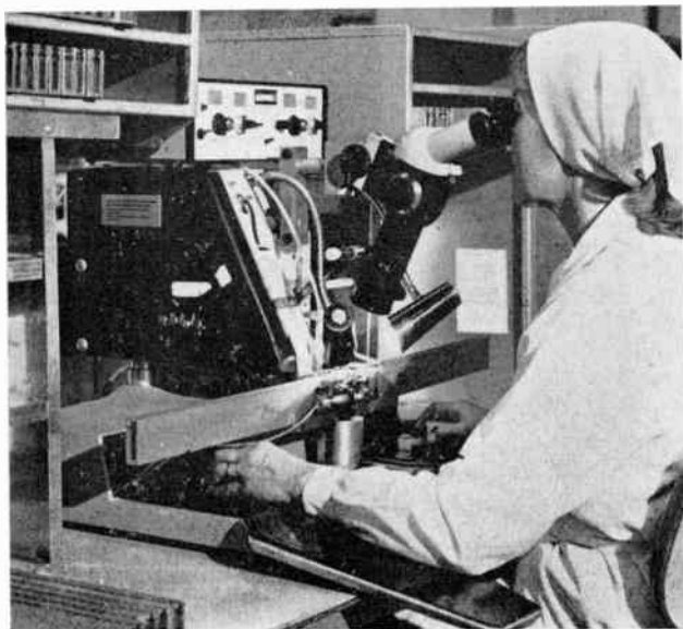
Fig. 6. Device lead wire bonding in assembly.
