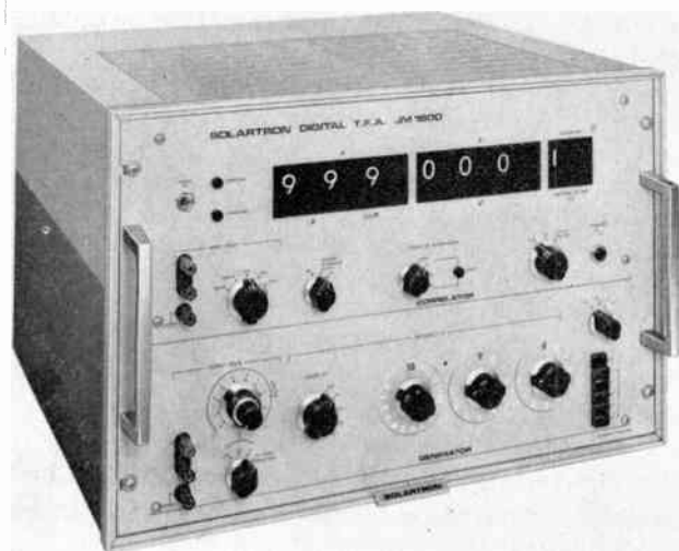
Fig. 5. Digital transfer function analyser containing over 700 transistors and 1900 diodes.
