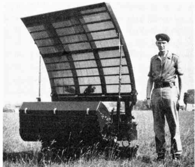
(b) Modern counterpart of (a). The reduction in power requirements allows the generator to be incorporated in the single unit.
