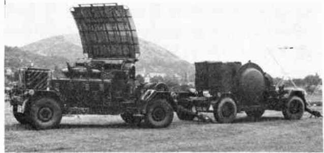
(a) Mortar locating radar with its power generator on a separate trailer.
