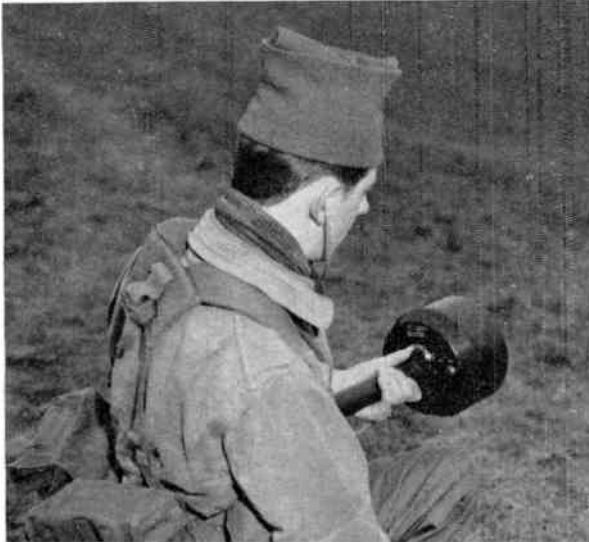
Fig. 6. The Small Portable RADar Torch (SPRAT) detects moving objects out to 1 km range by aural presentation of Doppler shifted echoes.
