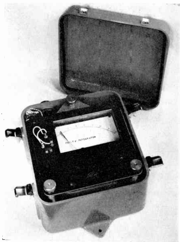
Fig. 11. The integrator in its cast-iron box with the drip-proof lid removed.
