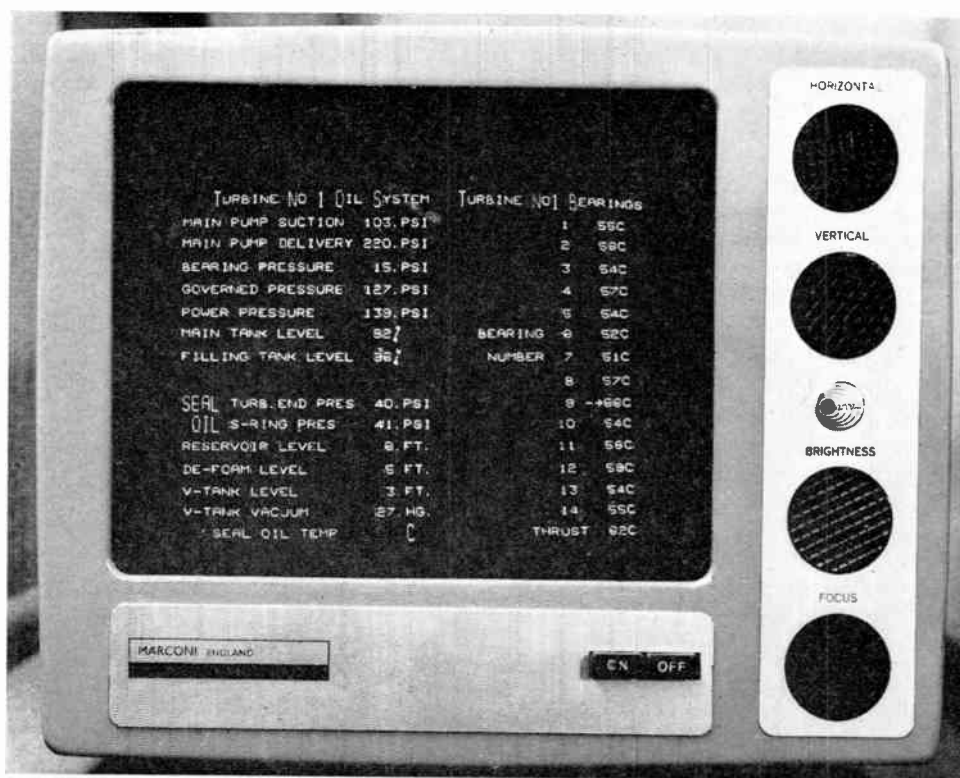
Fig. 7. Alpha-numeric display of processed information on cathode-ray tube.
