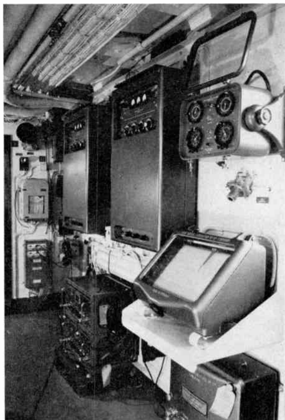
Fig. 4. Chart room housing receivers, display units and track plotter. The Decometer unit has upper meters indicating fine pattern readings ( 24f and 36f ). Whole lanes and lane identification are given by the lower dials.
