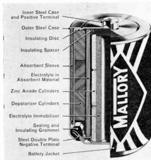
Cut-away view of the manganese battery. The manganese "cathode" is distributed in the depolarizer cylinder mix.
