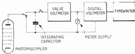
Fig. 2. Schematic diagram of direct reader measuring circuit.
