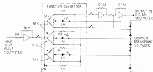
Fig. 7. Circuit to simulate a complete curve.
