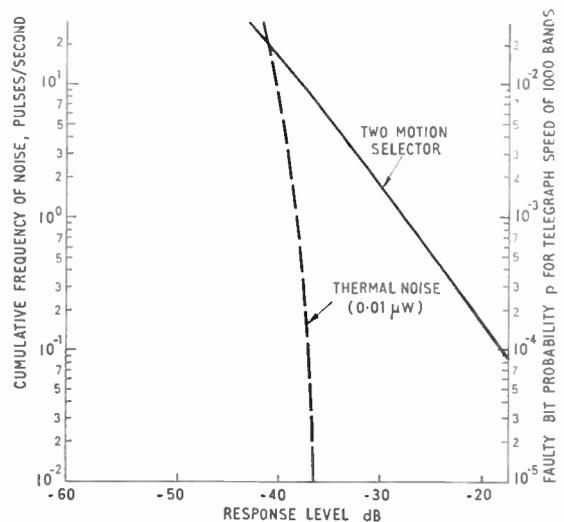
Fig. 2. Cumulative frequency distribution of noise pulses.
