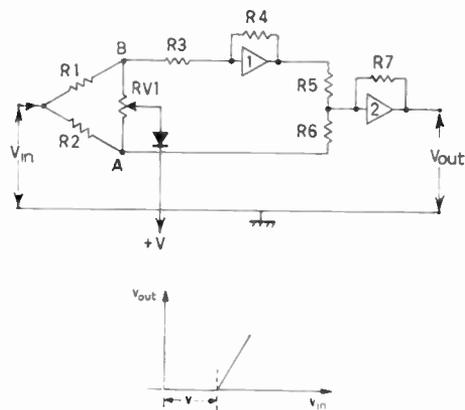
Fig. 6. Circuit of single segment and its characteristics.
