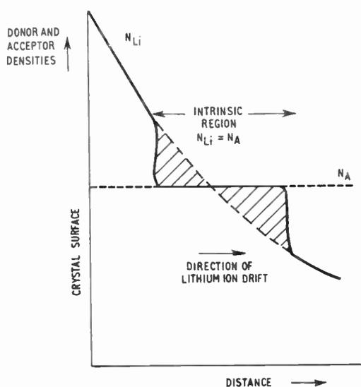
Fig. 4. Ion density distribution during the lithium ion-drift process.  $N_{Li}$  is lithium ion density,  $N_A$  the initial density of acceptor ions.
