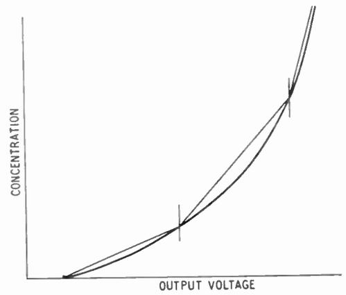
Fig. 5. Multi-segment approximation to calibration curve.
