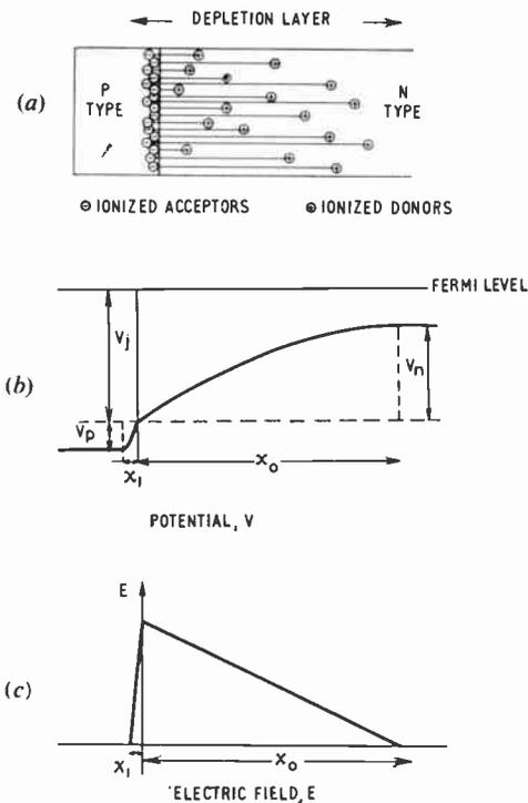
Fig. 3. Potential and field distribution in the depletion layer of a *p-n* junction.
