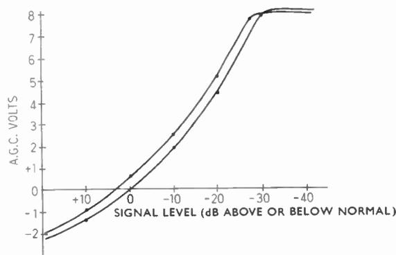
Fig. 11. Typical a.g.c. characteristic curves.
