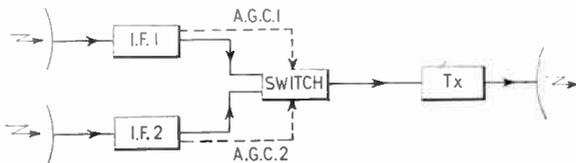
Fig. 5. Dual space diversity block schematic.
