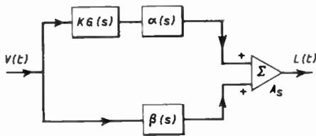
Fig. 3. Schematic diagram of transportation lag unit.
