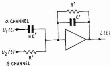
Fig. 4. The summing amplifier,  $\alpha(s)$  and  $\beta(s)$  functions.
