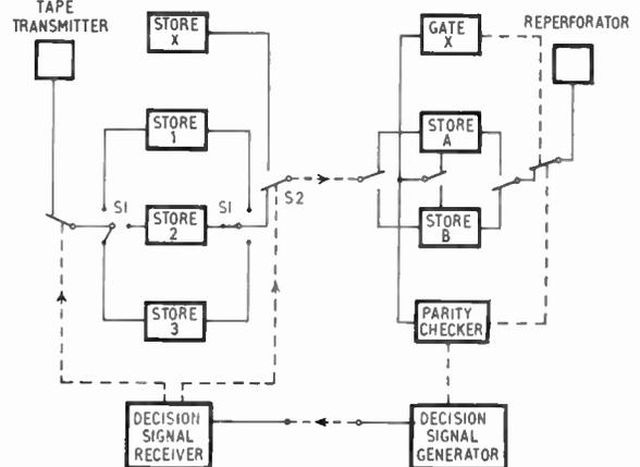
Fig. 5. Block layout of an error detection and correction equipment for use on the telephone network.
