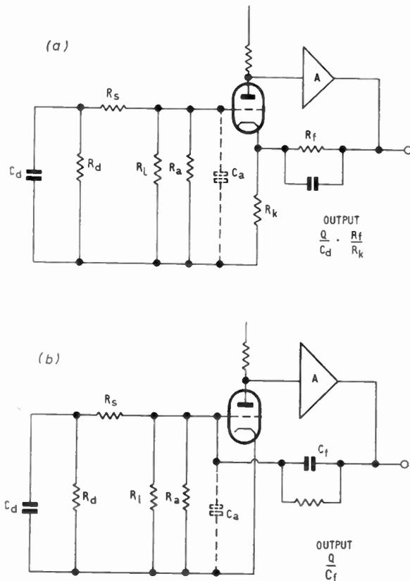
Fig. 7. Input circuit parameters for (a) a voltage-sensitive and (b) a charge-sensitive amplifier configuration.
