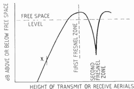
Fig. 3. Variation of received carrier level with height of transmit or receive aerials.
