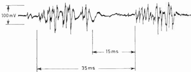
Fig. 1. Typical noise burst on a telephone circuit.
