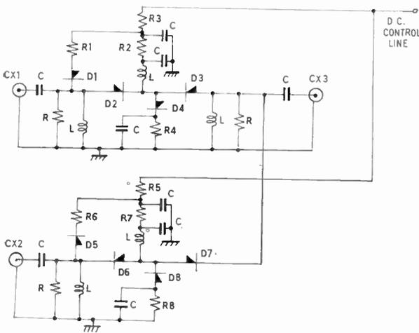
Fig. 8. Schematic diagram of diode switch.
