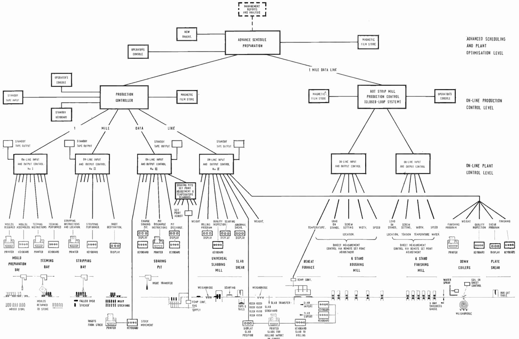
Fig. 3. Hierarchy system for steel strip mill.
