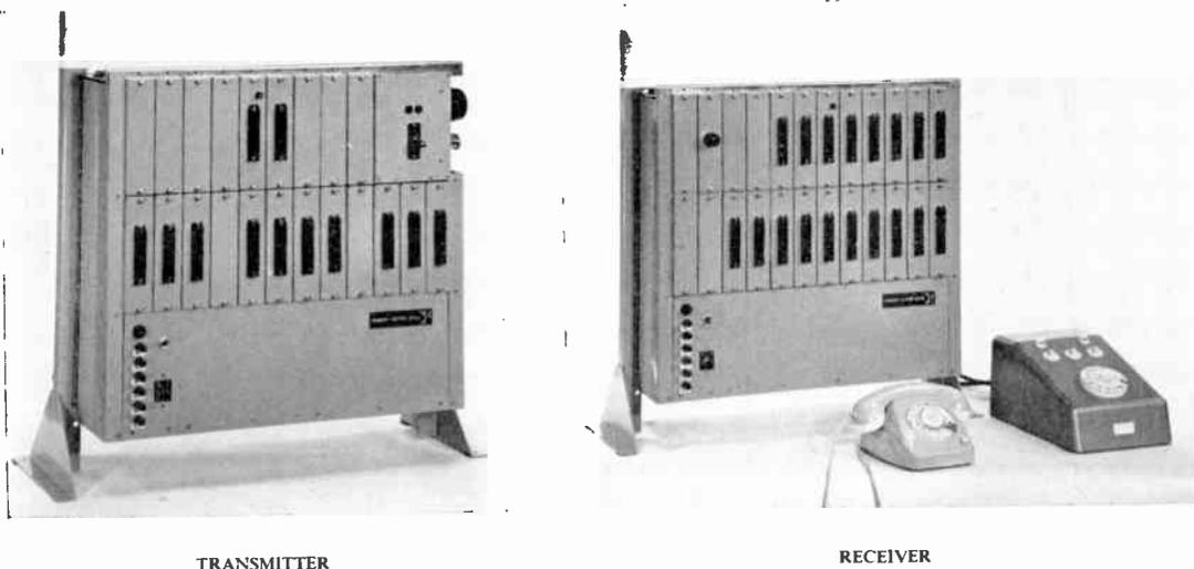
Fig. 6. Experimental data transmission system with automatic error correction by block retransmissions.
