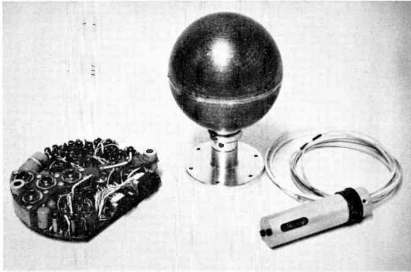
Fig. 3. Gridded sphere and circuitry for determination of ion mass spectrum and temperature.
