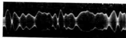
Fig. 6. Reverberation plus a single target echo at the output of 100 c/s filter.
