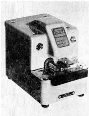
Fig. 1. The high-speed tape reader. (a) External and (b) internal views.
