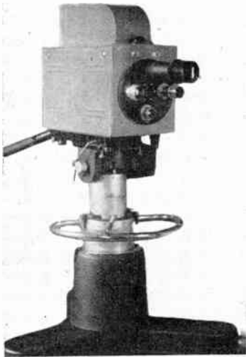
Fig. 2. An image orthicon camera for outside broadcasts. The controls placed below in the rear part of the camera serve for lifting and lowering the mount (when the camera is installed on a special mount) and for optical focusing. The position of controls facilitates the operator's work during panning shots.
