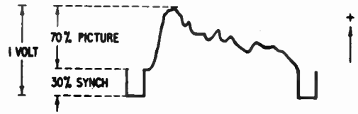
Fig. 1. Form of signal at a video point.
