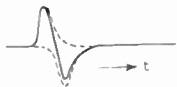
Fig. 2. Playback waveform of a short rectangular pulse. The positive - and - negative - going components are shown dotted.
