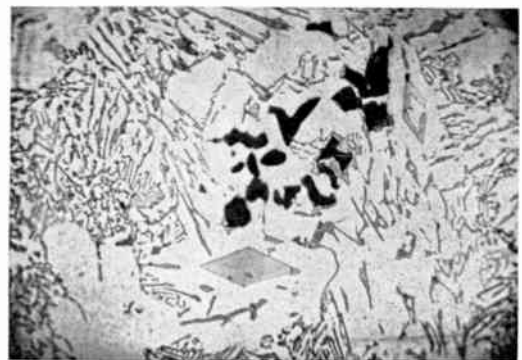
Fig. 4. Uranium-aluminium alloy (Magnification \times 3000 on screen).
