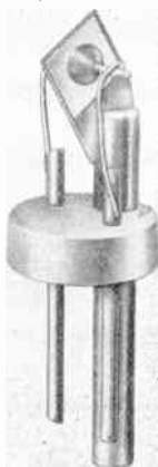
Fig. 1. (a) Switching transistor design. (b) Switching transistor from laboratory production.
