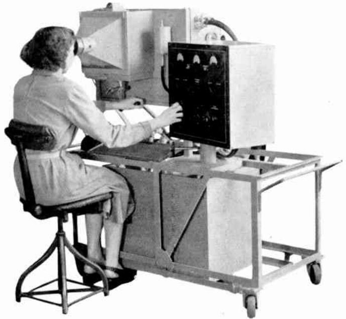
Fig. 1.—A 150-kV mobile fluoroscopic x-ray unit.
