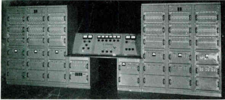
Fig. 3.—Analogue computer for the investigation of aircraft flutter.
